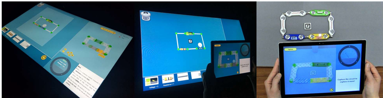
Figure 2. Three different version of our design: a single-display version (left), an AR version (middle), and a tangible version (right)
