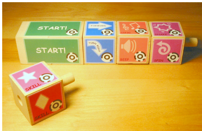
Figure 1. A tangible programming language for robotics developed at Tufts University. With this language, children construct programs using interlocking wooden blocks.
