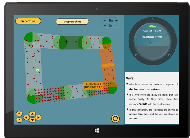
Figure 4. Electron model display in the AR condition. The blue dots are moving electrons and the red dots represent ions in conductive materials. Resistors have higher ion densities than wires.
