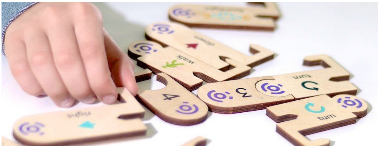
Figure 22.1 A prototype tangible programming language based on computer vision technology.
