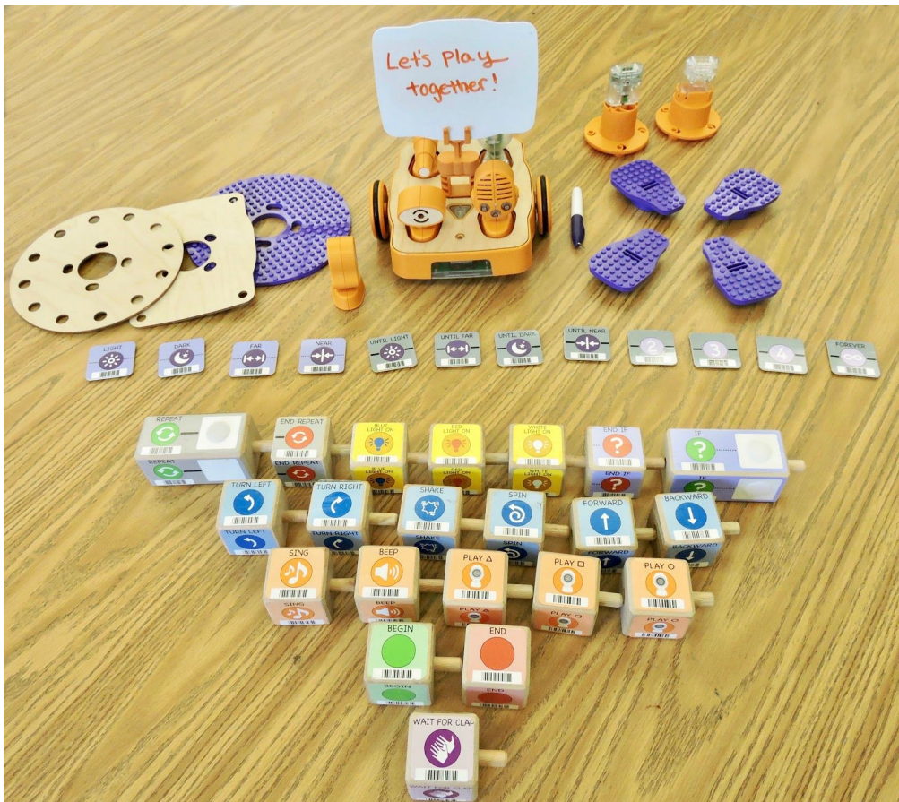
Figure 22.2 KIBO robot and its blocks. Reproduced with permission from Bers (2018b).
