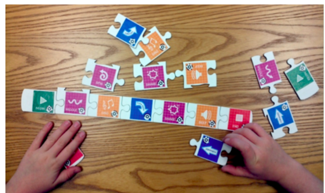
Figure 2: The Tern tangible programming system uses puzzle pieces for the physical construction of computer programs.
