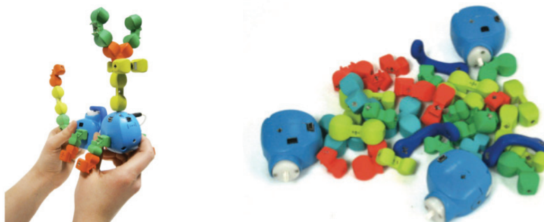
Figure 1. A Topobo Moose (left): to program motions, you just manipulate the toy; and Topobo pieces (right).
